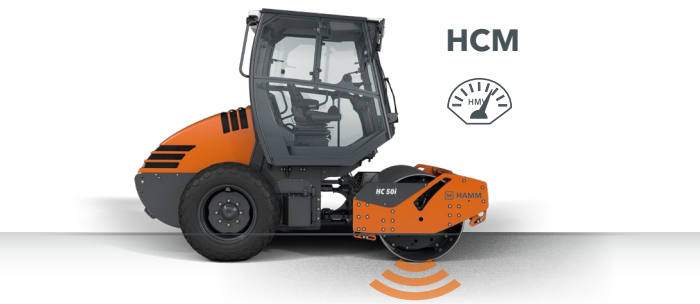
Thanks to their even weight distribution, the compactors have high traction, even on rough terrain.
